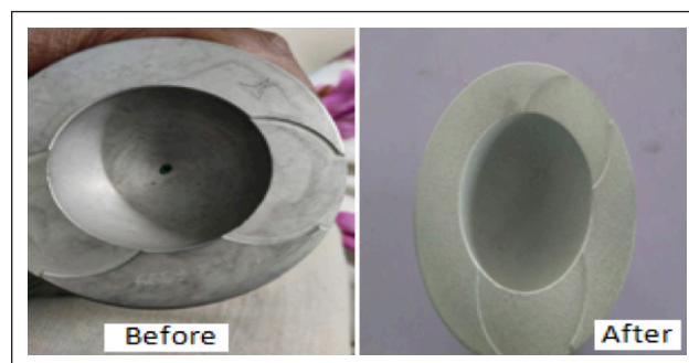
Figure 2. Piston before/after coating.
