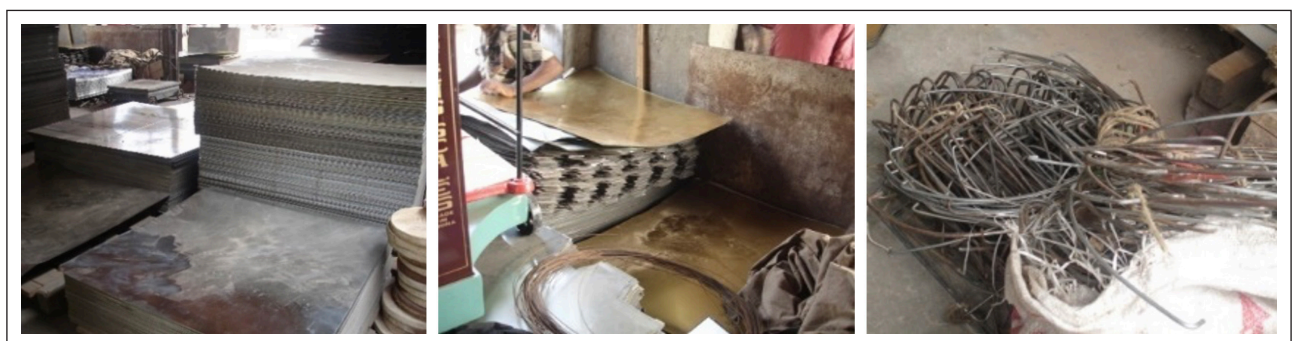
Figure 8. New metal sheets, old and cut sections of metal sheets, metal handles of rejected buckets (left to right).
