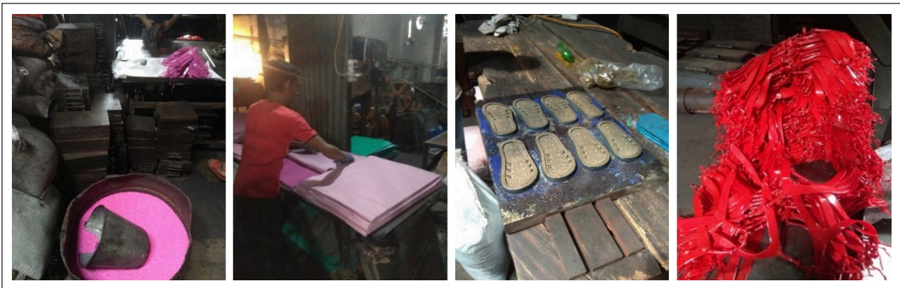
Figure 13. EVA raw material for producing rubber sheets, newly produced rubber sheets, dice for preparing shoe sole and newly produced PVC sandal straps (left to right).
