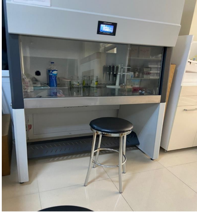
Figure 2. Biosafety cabinet and chair for the microbiology laboratory
