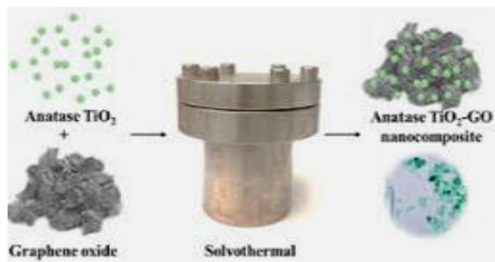
Figure 9: Synthesis of Nanoparticle using Solvothermal Method (24).
