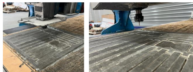
Figure 5. The cutting samples from composite plates with CNC router
