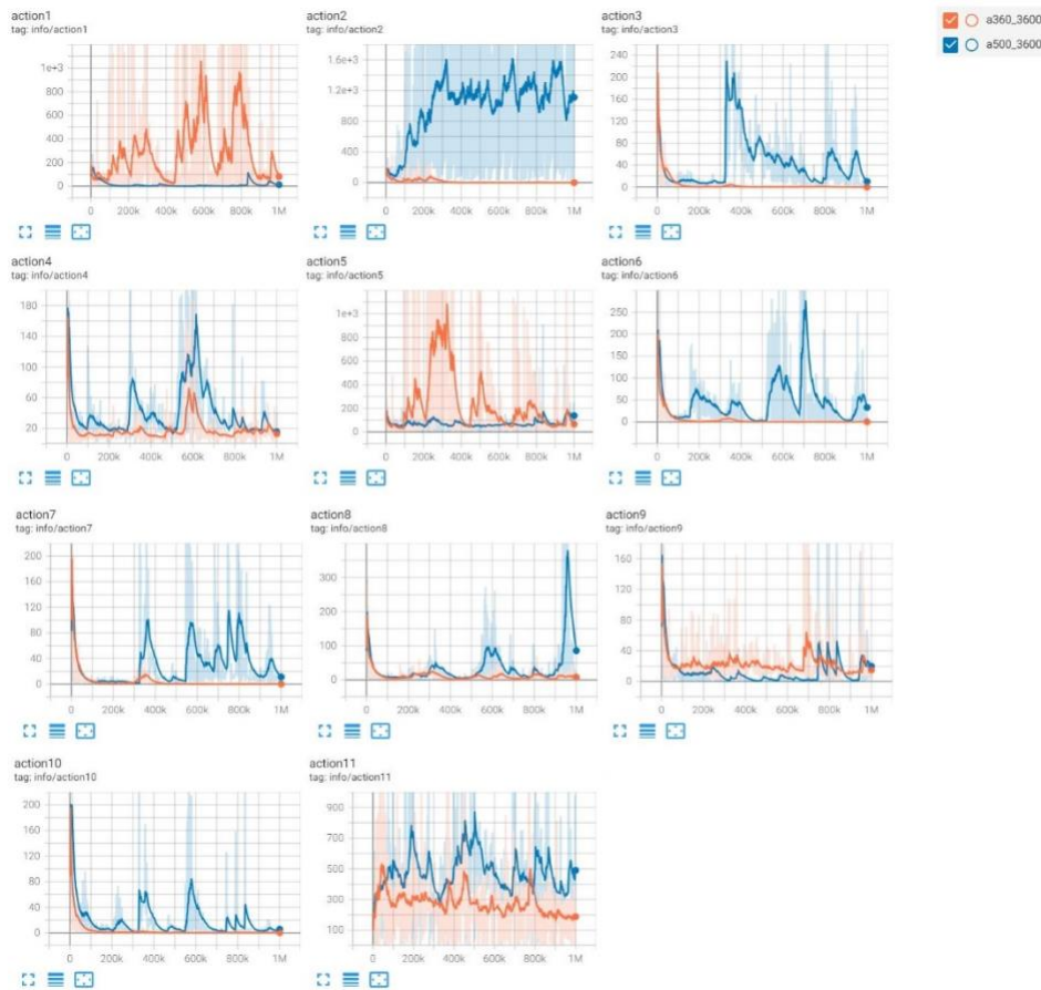
Figure 6. The mean number of actions executed per episode for different order throughputs during training for 1 hour arrival interval
