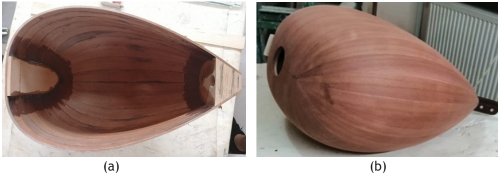
Figure 6. The bowl of baglama made by gluing wood pieces together (a) Inside view (b) outside view
