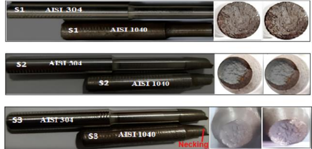
Figure 14. Tensile test broken pictures of samples S1, S2, and S3
