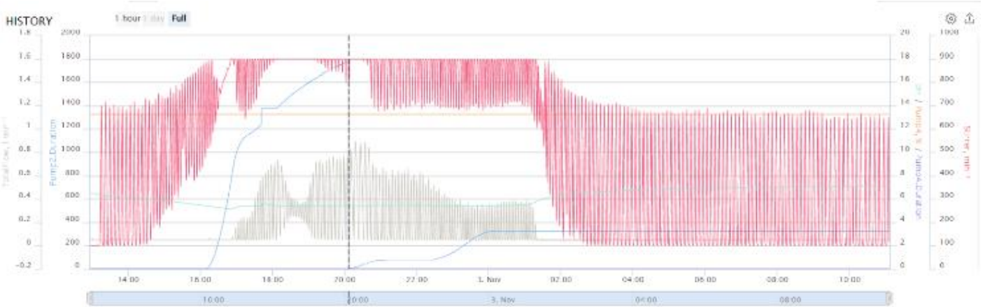
Figure 3. The evolution of pO 2 , pH, agitation, temperature, base pump duration over time. The graph shows the pH level (blue), stirrer (pink), base pump duration (dark blue), total flow (grey).
