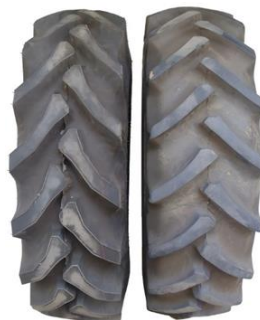
Fig 4. Test tires used in the study, a-) Bias, b-) Radial
