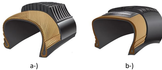
Fig 3. Different types of tires, a-) Bias-Ply, b-) Radial [14]
