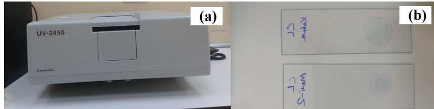
Figure 1: (a) UV-visible spectrometer used for optical absorption measurements of contact the lenses, (b) Examined lens samples
