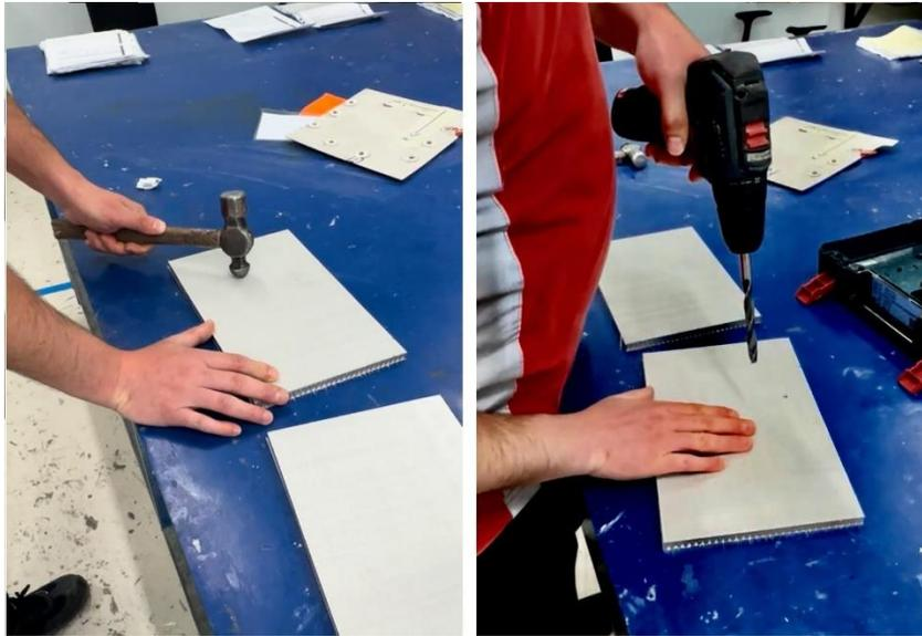
Fig. 5. Induction of artificial damage on the samples.
