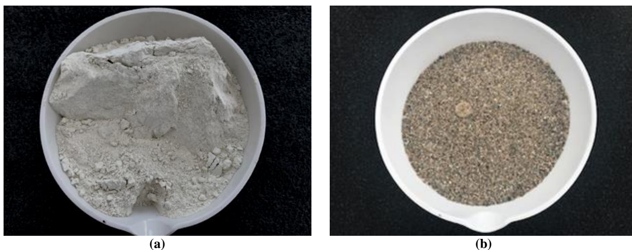
Figure 1. Soil types used in the testing program: (a) Bentonite clay, (b) Beach sand
