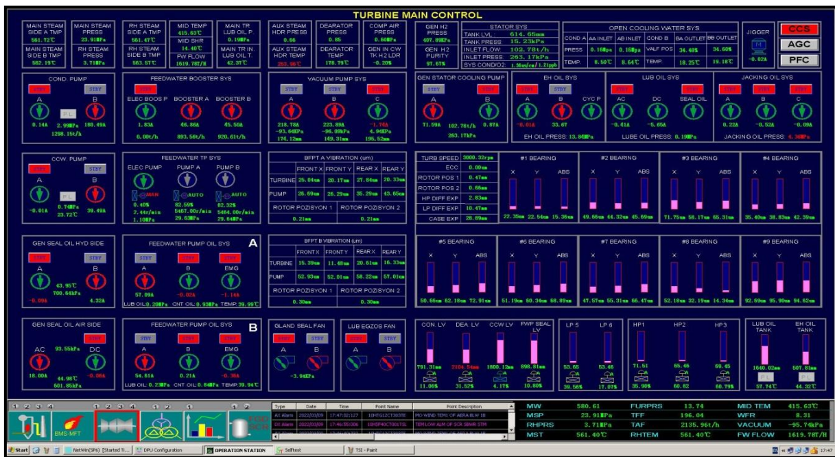
Figure 2. Distributed Control System (DCS)
