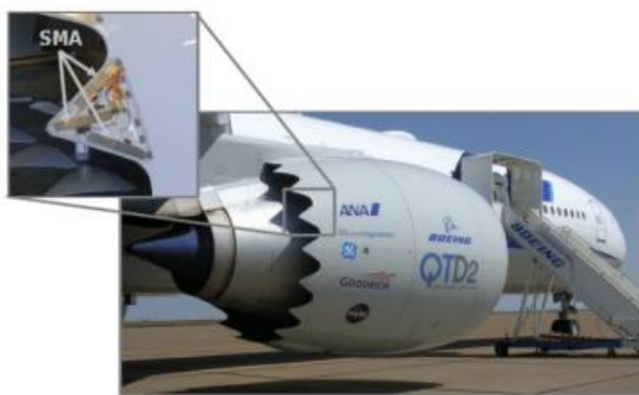
Figure 1. SMA application on Boeing's variable geometry chevron (Costanza & Tata, 2020).
