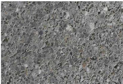
**Figure 9.** Polymer Concrete [30]
