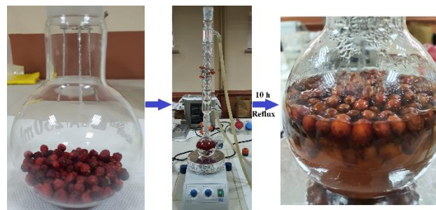
Figure 3. Schematic of Pyracantha coccinea berries extraction procedure
