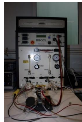
Figure 4. The PEMFC's MEA testing system
