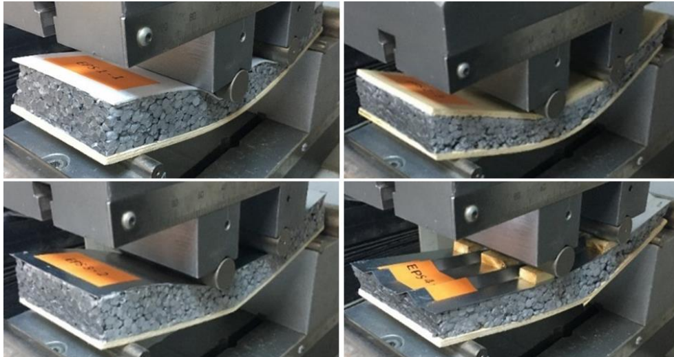
Figure 3. Four-point bending tests of EPS specimens
