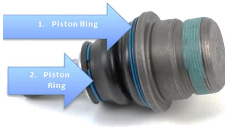
Figure 1. Representation of the piston rings in the tie rod end
