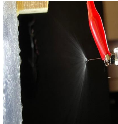
Figure 4. Electro spray generation
