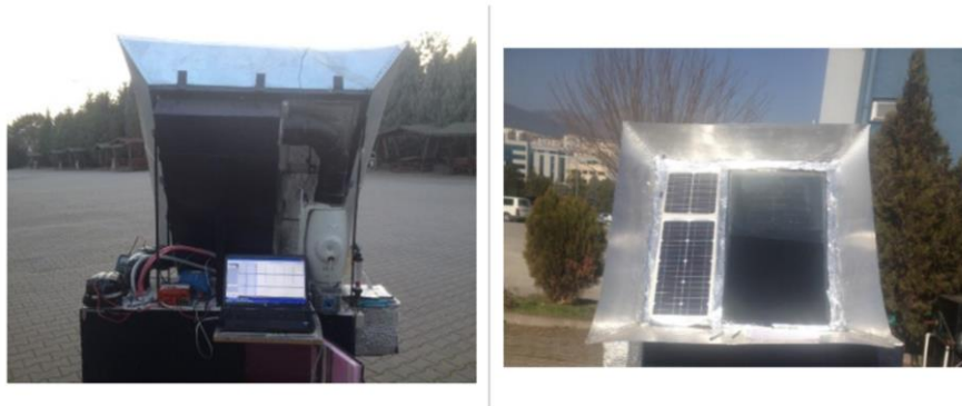
Figure 2. Indirect solar-powered drying system: (a) rear view, (b) front view
