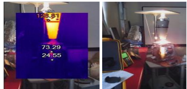
Figure 4. An image of the infrared lamp experimental level taken with a thermal camera
