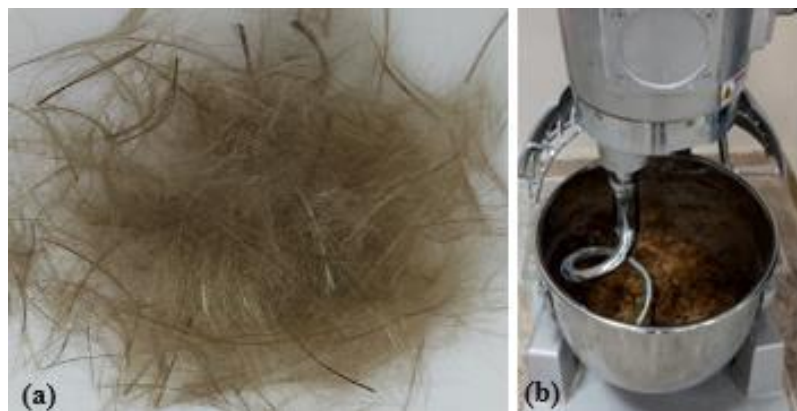
Figure 3. Separated BF used in the study (a) and preparation of mixtures (b)
