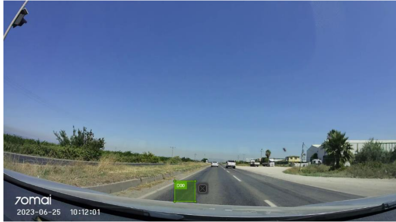
Figure 6. The ultimate annotated image comprises of bounding boxes and a class label, which in this instance is denoted as D00
