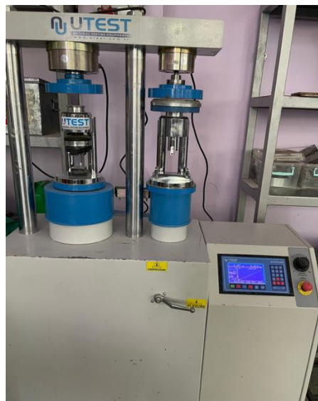
Figure 5. Three-point flexural test
