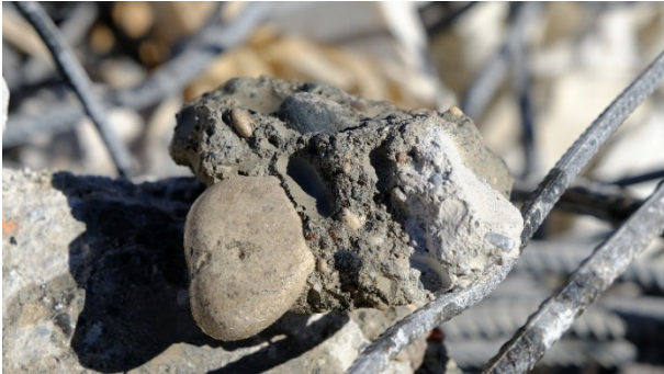
Figure 16. Aggregate that is not suitable in size and shape.
