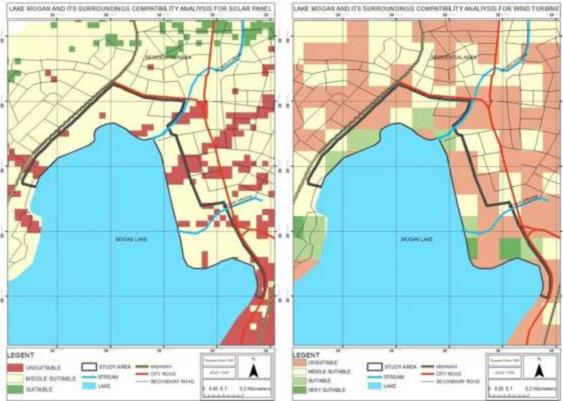
Figure 13. Suitability analysis for solar powered urban furniture and urban features (left), suitability analysis for wind powered urban furniture and urban features (right).
