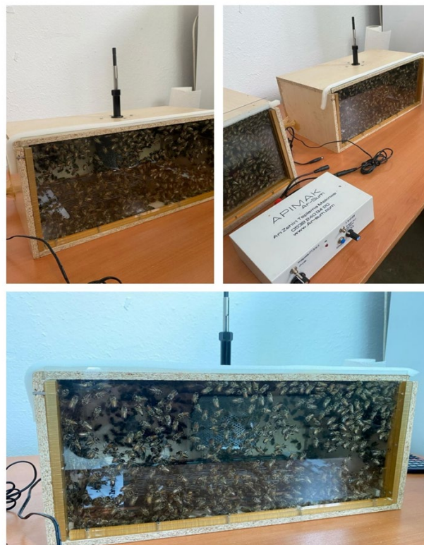
Figure 1. Special hive system for bee venom volatile analysis
