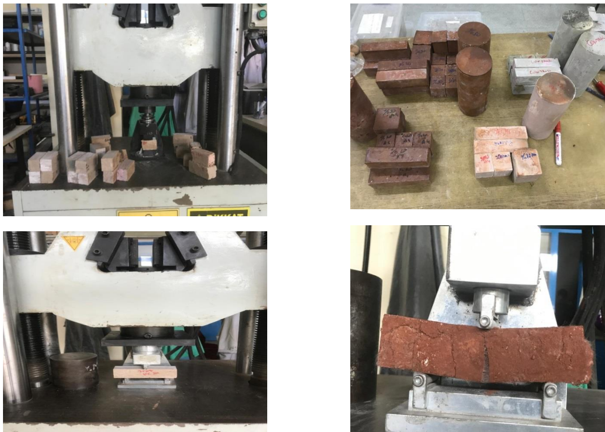
Fig. 1. Images of the experimental setup and specimen testing process, including preparation, testing, and storage of AACs.
