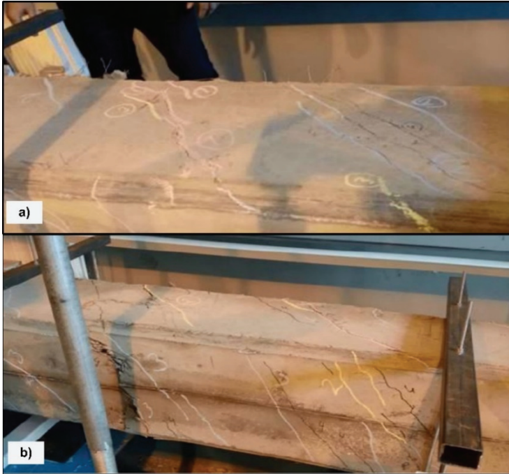
Figure 9 - Crack pattern of S30V15 (a) and S40V12 (b) beams
