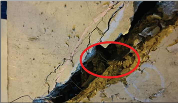
Figure 11 - The rupture of transverse reinforcement (S30V09 beam)
