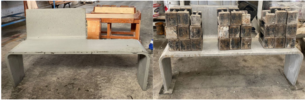
Figure 3. Shows the prototype product extracted from the mould on the left, and the physical loads applied to it on the right.
