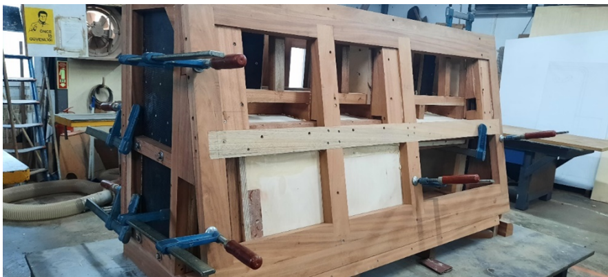
Figure 2. Wooden mould prepared for prototype casting.
