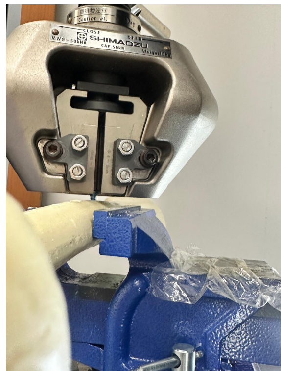
Figure 2. The installed system to test the prepared models. While the synthetic femur was affixed within the device, the head of the screw on the bone was grasped with the aid of a tool, and a tensile force was applied to the cortical screw head until pull-out (load to failure)
