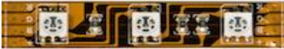
Figure 2. SMD 5050 RGB LED chip (left) and RGB LED module (right).
