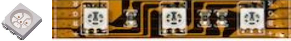
Figure 2. SMD 5050 RGB LED chip (left) and RGB LED module (right).
