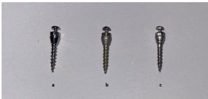
Figure 1. a) CNC Titanium (CNC-T), b) SLM Titanium (SLM-T), c) SLM Stainless Steel (SLM-SS) mini-screws.
