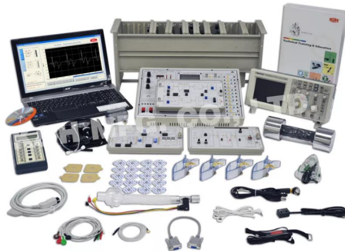
Figure 1: Biomedical Measurement Training System KL-75003 [10].
