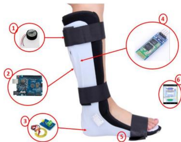
Figure 3: The Hardware Components of the Developed Orthosis
