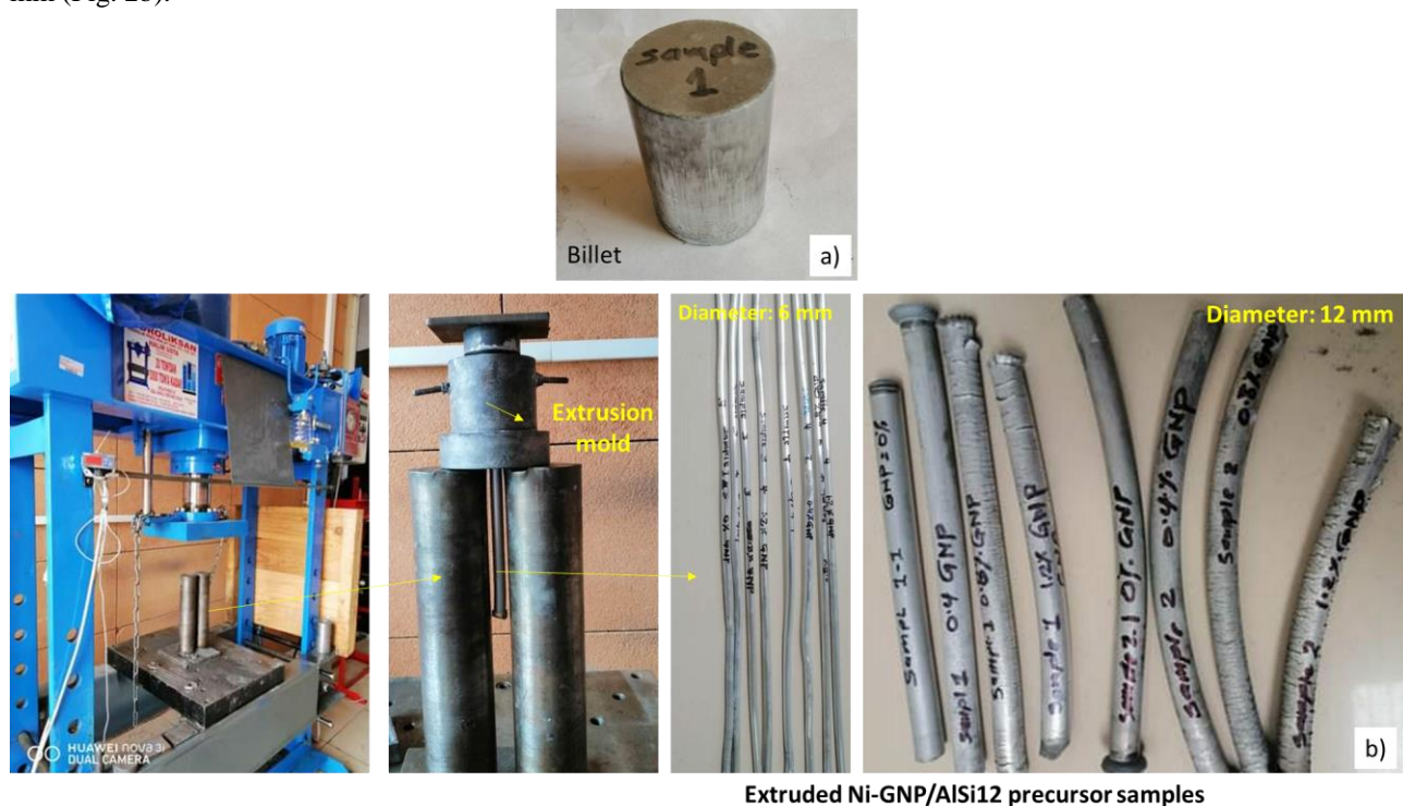
Figure 2. Compressed block sample (billet) (a) and extruded Ne-GNP/AlSi12 precursor samples
