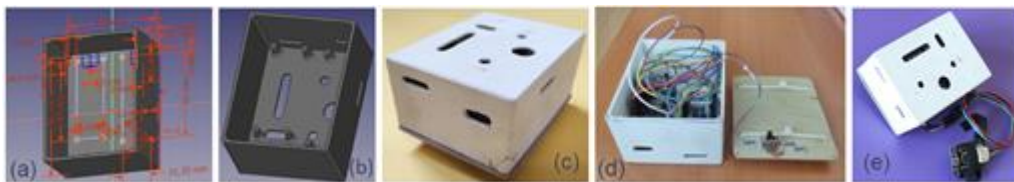
Figure 4 (a) Design with dimensions (b) 3-D view without dimensions (c) Design printed with white plastic (d) Modules installed in the case (e) Heart Rate and Oximeter Sensor connected.
