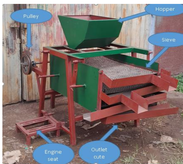
Figure 5. Pictorial view of the developed grading machine.
