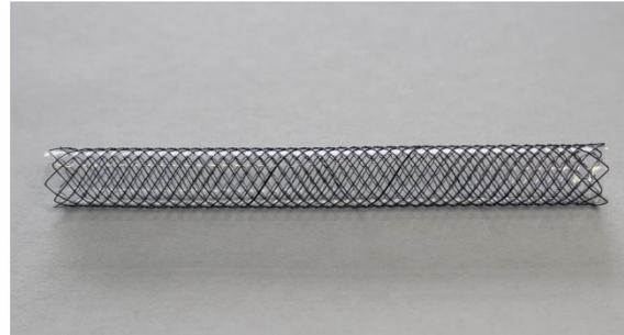
**Figure 5.** Traditionally manufactured 316l steel stent.
