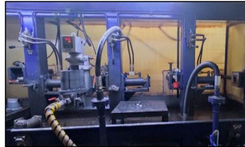
**Figure 3.** Pump efficiency test unit.
