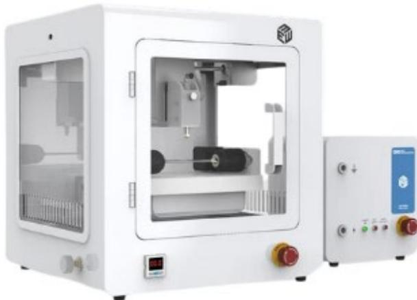
**(A) Melt Electro Writing Device**
