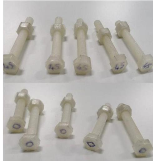
**Figure 4.** PLA Bolts and Nuts Samples
