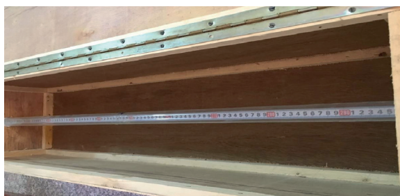
Figure 2. Chemotropism device used in testing the repulsive and attractive properties of mint essential oil and mint methanol leaf extract
