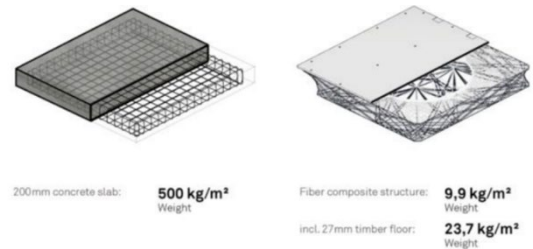
Figure 6. ICD/ITKE 2021 Pavilion, comparison of reinforced concrete slab vs lightweight slab (Menges & Dambrosio, 2021).
