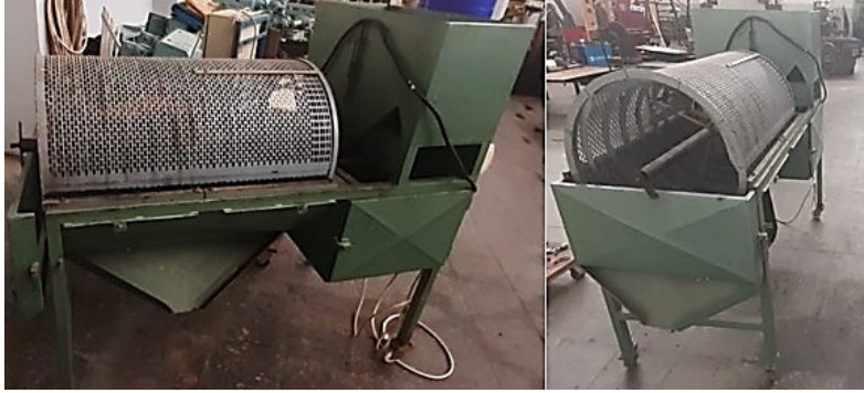
Figure 1. The peanut grading (sorting, sieving, classification) machine used in the experiments.
