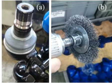
Figure 3. Process Faults and Cleaning Brush (a) A Fail in The Painting Process (b) Cleaning Brush
