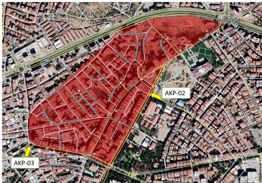
Figure 2. Akpınar DMA network layout [19]
