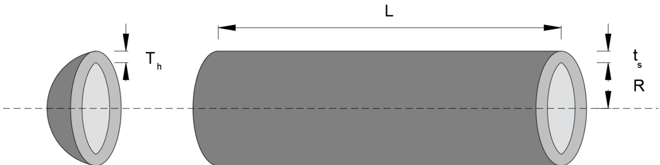
Figure 9. Schematic representation of pressure vessel design problem
