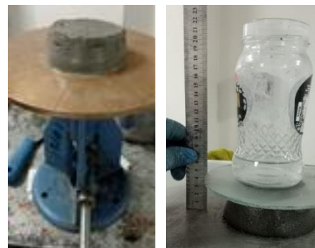
Figure 3. The buildability test GP mortar sample.
