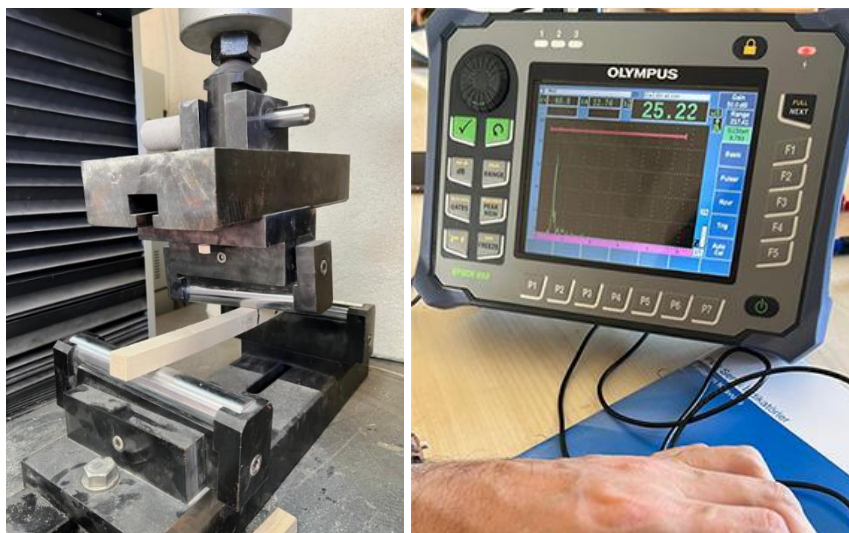
Figure 2. 3 points bending test (left) and ultrasonic measurements (right)
