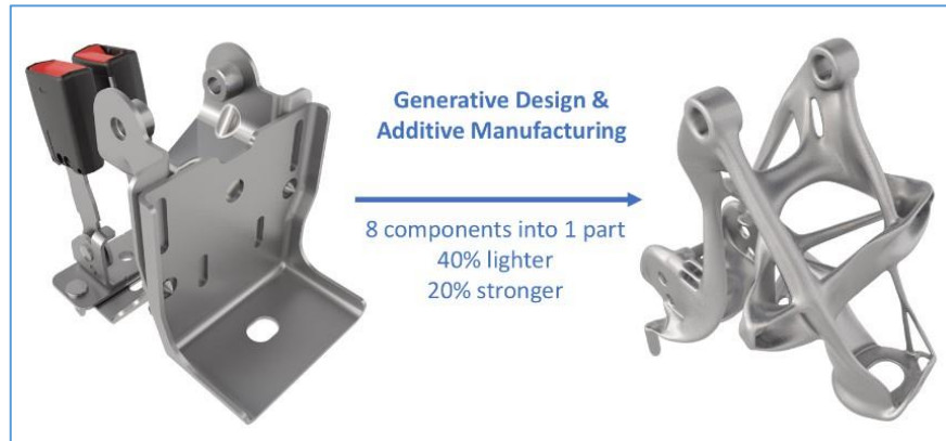
Figure 3. The example of seat bracket designed using Generative Design [18].
