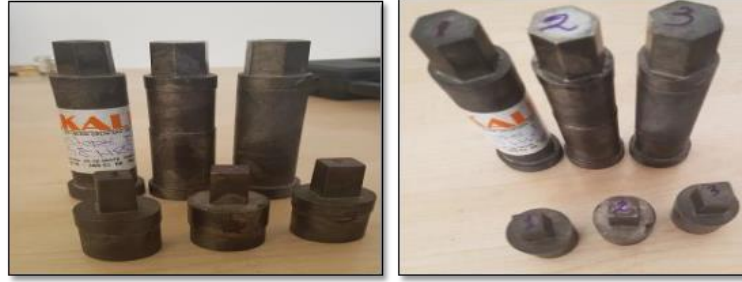
Figure 2. The types of three punch sets (Üçlü zimba setleri)
