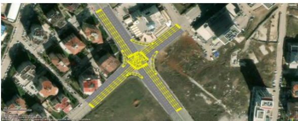
Figure 7 Intersection design calibrated for no lane changes: each lane as a separate link.
