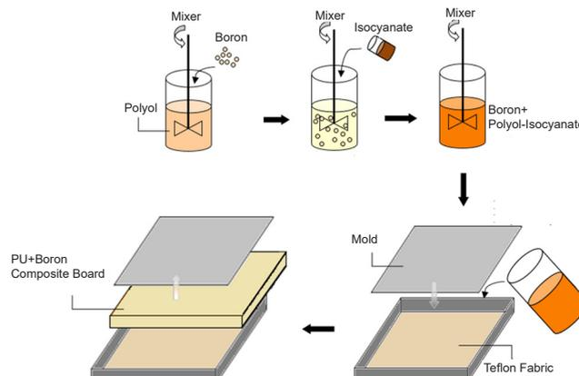
**Figure 1.** Production process of the composite board
