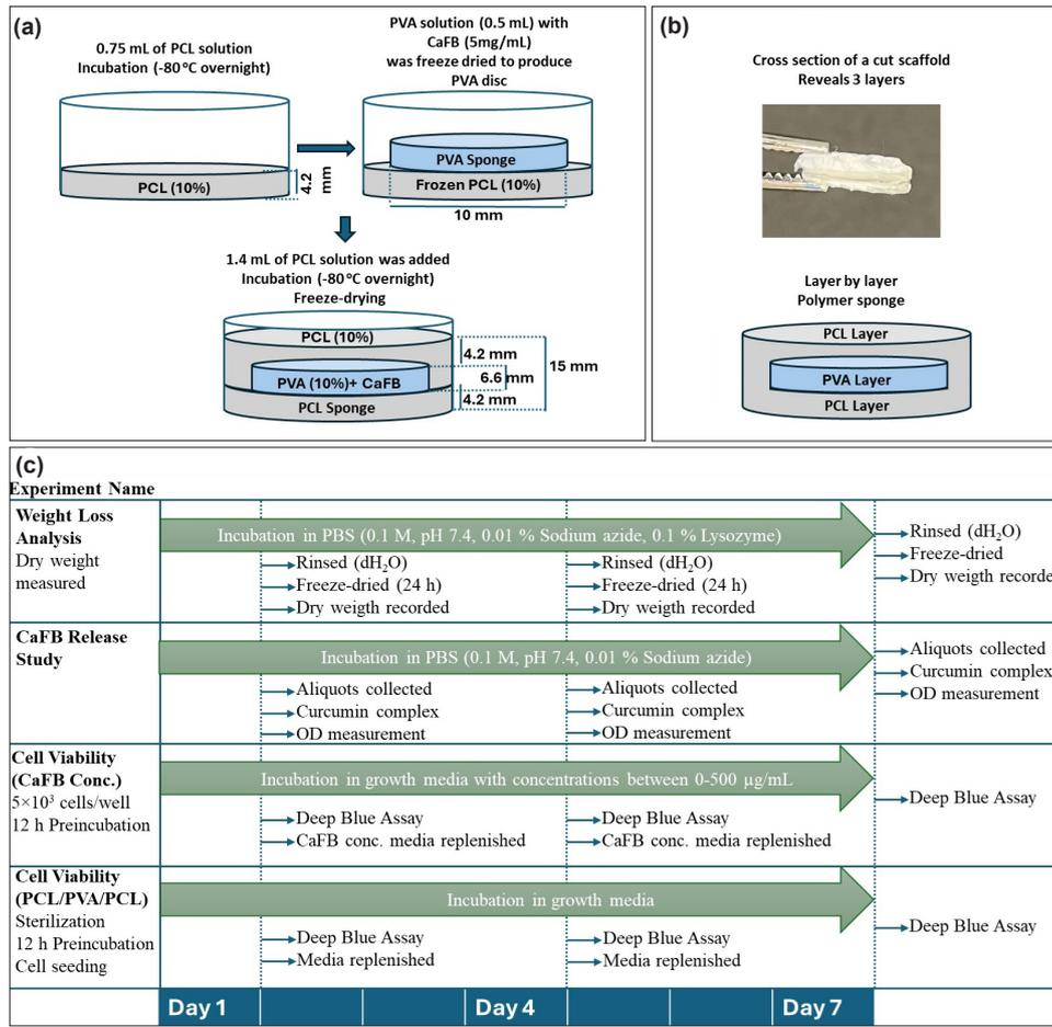
**Figure 1.** a) Schematic representation of the layer-by-layer scaffold fabrication via freeze drying method. b) Cross section of the PCL/PVA/PCL scaffold and schematic representation of the final form of the layer-by-layer scaffold. c) Diagram showing the experimental steps performed at incubation time points
