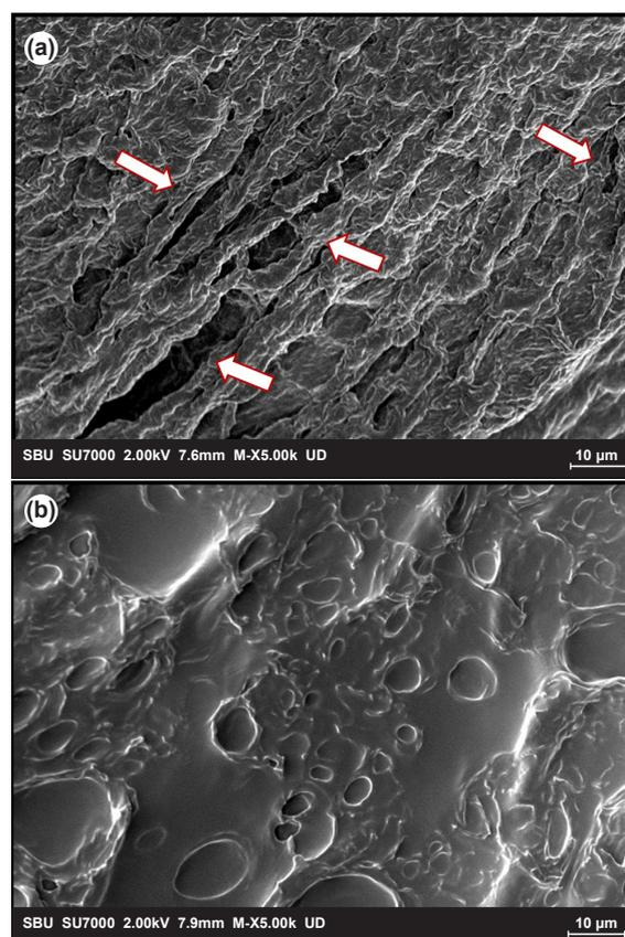
**Figure 2.** FE-SEM images of scaffold layers, PCL (a) and PVA (b). Arrows show the pores that have been created on the surface. Images were taken at 5000X magnification and scale bars show 10  $\mu$ m length
