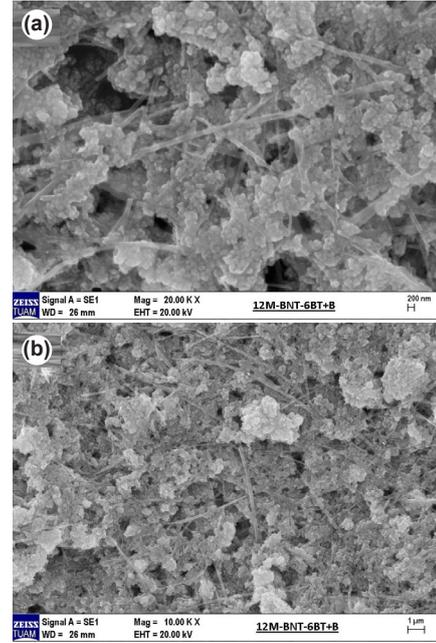
**Şekil 2.** 20.000X (a) ve 10.000X (b) 12M NaOH çözeltisi ile üretilen BNT-6BT+ %1 mol B<sup>3+</sup> tozunun SEM görüntüleri (Ölçek çubukları a) 200 nm, b) 1 µm). (20,000X (a) and 10,000X (b) SEM images of BNT-6BT+1 mol % B<sup>3+</sup> powders synthesized via hydrothermal method with 12M NaOH solution (Scale bars a) 200 nm, b) 1 µm)
