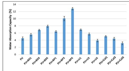
**Figure 9.** The water absorption capacity of PU and its composites
