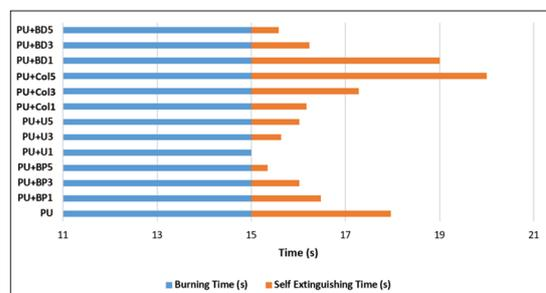
**Figure 7.** Self-extinguishing times of PU and its composites
