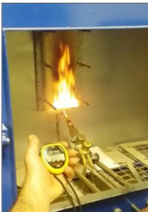
Figure 2. Ignitability test
