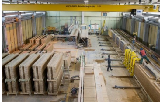
Figure 5. Lehm Ton Erde LLC Company in Austria Prefabricated Manufactured Rammed Earth Wall Practices (Rauch, 2020:2)
