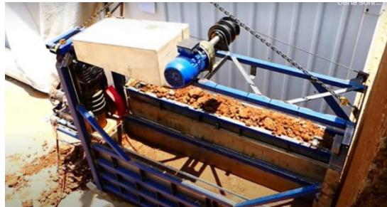
Figure 6. Sliding Mould System of Form Earth© Company in Australia (Url-2).
