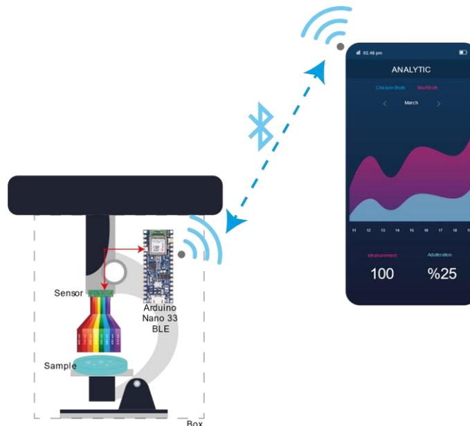
**Figure 1.** The mobile spectral setup
