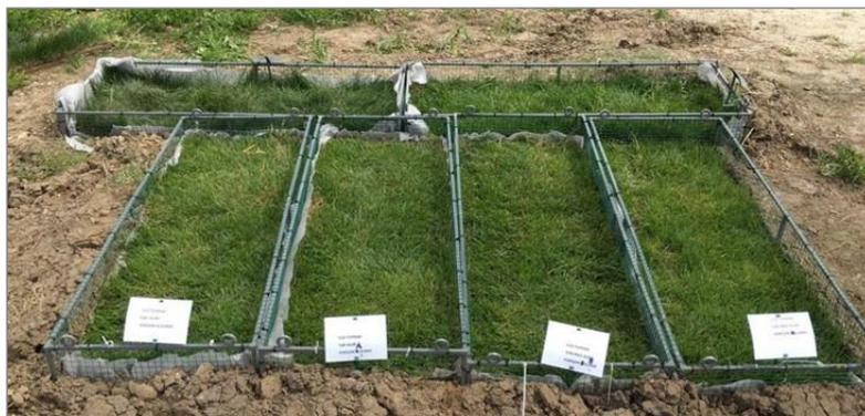
**Figure 3.** Basket with a size of 1.3m x 0.5m x 0.2m in which rootzones were placed
