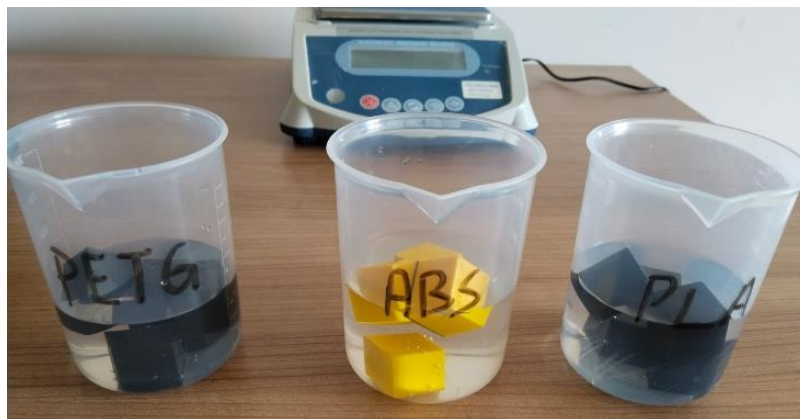
Figure 10 Weighing the samples by keeping them in pure water
