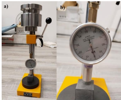
Figure 6 a) Shore Durometer NOVOTEST TS-A hardness tester, b) zeroing the load scale
