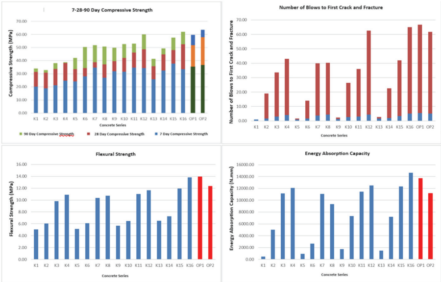
Figure 14 - Experimental results for optimization and Taguchi series
