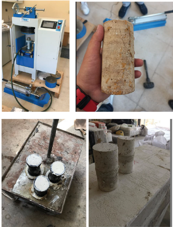
Fig. 3 - Triaxial pressure system and prepared samples for experiment.
