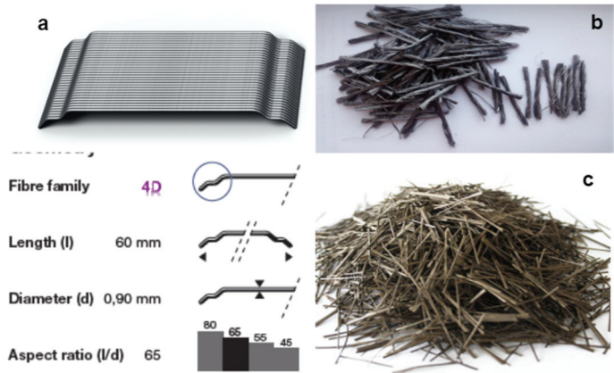
Figure 2 - The fibers used in concrete; a) steel fiber, b) polypropylene fiber, c) basalt fiber.
