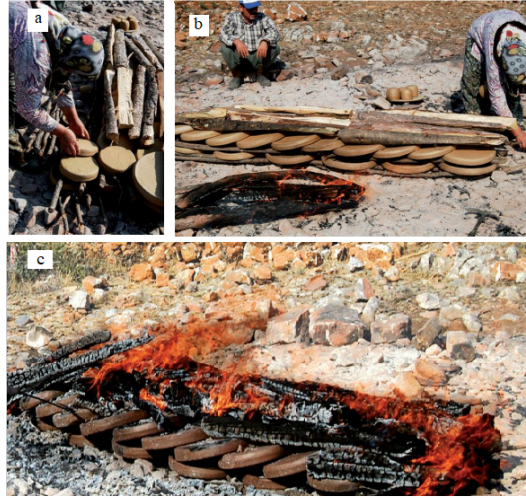
Figure 2: Open firing process in Sorkun [17].
