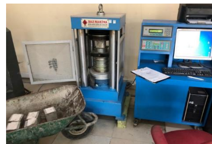
Figure 4. Compressive strength measurement device
