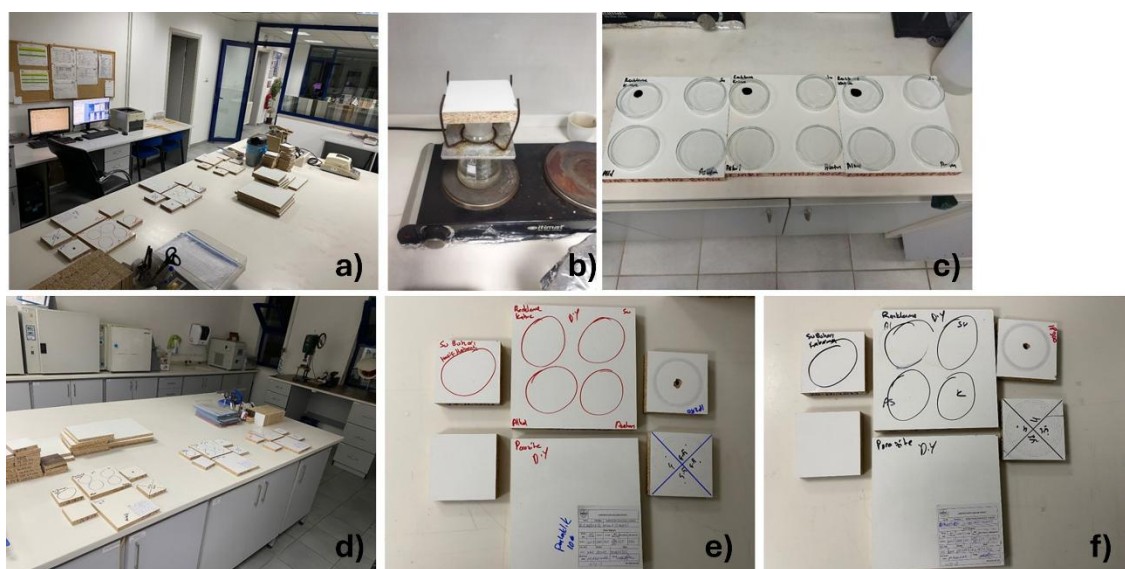
Figure 1. The standard tests for staining resistance quality check in laboratory conditions (a: Test laboratory, b,c: Treatment process, d,e,f: Analysis process)
